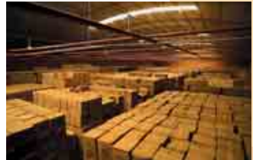
Multi-level storage on slabs. Uniform loading max of 5 t/m 2 . Max allowable differential settlement: 0.8/1000.
